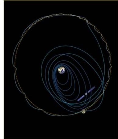
Fig.1b: SMART-1 spacecraft trajectory spiralling out from Earth
