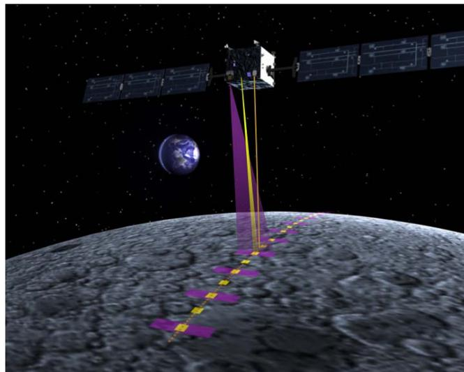
Fig. 10: Comparison between the swaths of the SMART-1 remote sensing instruments in lunar orbit: D-CIXS (32 x 12 deg), AMIE (5x5 deg or 2.5x1.25 deg colour frames) and SIR (4 arcmin point spectral continuous mapping)
