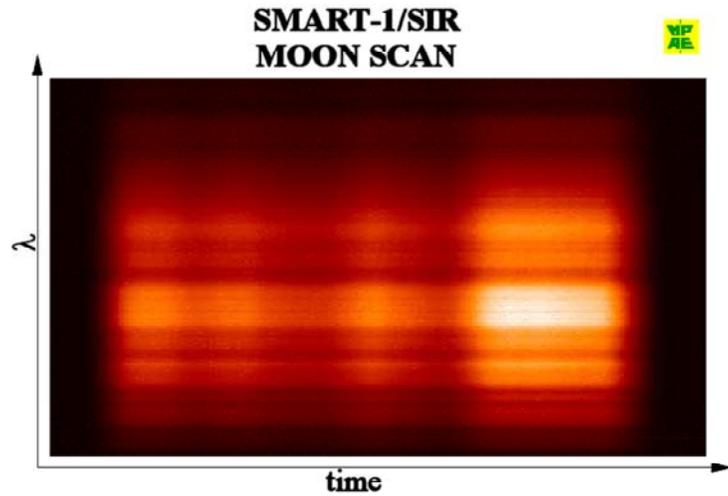
Fig. 5b: First SMART-1 spectra of the Moon obtained by scanning the SIR infrared spectrometer from limb to limb, showing lunar regions of different albedo.
