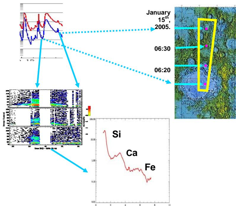
Fig.3: First SMART-1/ D-CIXS lunar measurements obtained during solar flare on 15 January 2005, when orbiting over Mare Crisium and near highlands. The spectra obtained from the three D-CIXS facets were summed over the duration of the flare, giving the spectrum showing chemical elements such as Silicon, Iron and Calcium for the first time from orbit. The elemental abundances were derived along the track, and compared in particular with samples from Mare Crisium returned by Luna 24.
