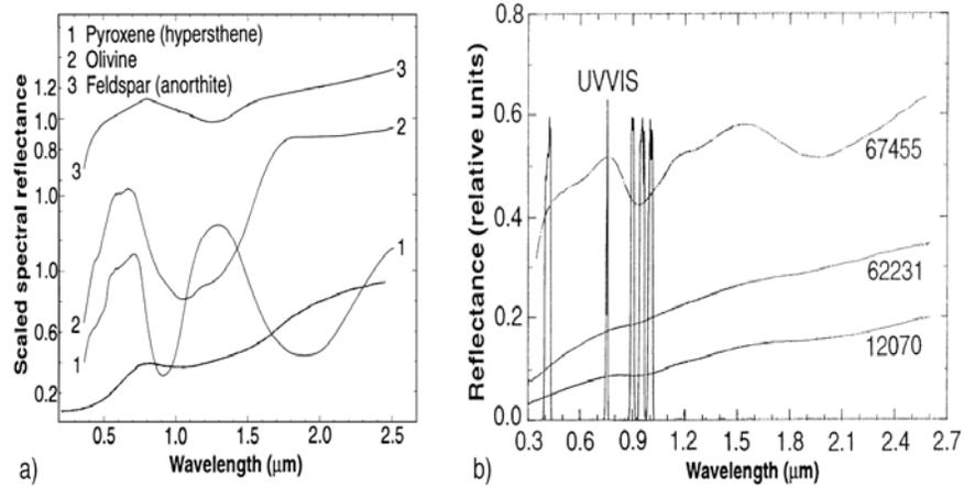
Fig. 5a: Reflectance spectra of key lunar minerals at UVVIS and NIR wavelengths (Courtesy of C. Pieters). The left hand plot shows the spectra of pyroxenes (1), olivines (2) and feldspar (3) while the middle plot shows reflectance spectra of lunar samples. The NIR measurements up to 2.4 μm provided by SIR allow for the separation of the mineralogical signatures. AMIE filters correspond to 0.75, 0.9, and 0.96 μm.
