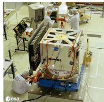
Fig.1a: SMART-1 spacecraft during integration and functional tests (<http://sci.esa.int/smart-1/>)
